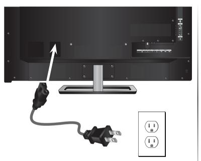
Connect the power cord to the back of the TV. Plug the power cord into an electrical outlet.
